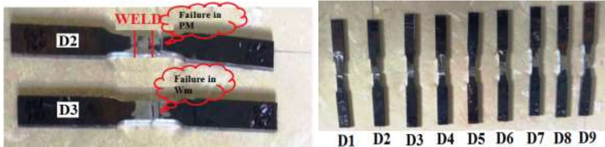
Figure -4.3 Tensile Test Specimens Before and After Test
