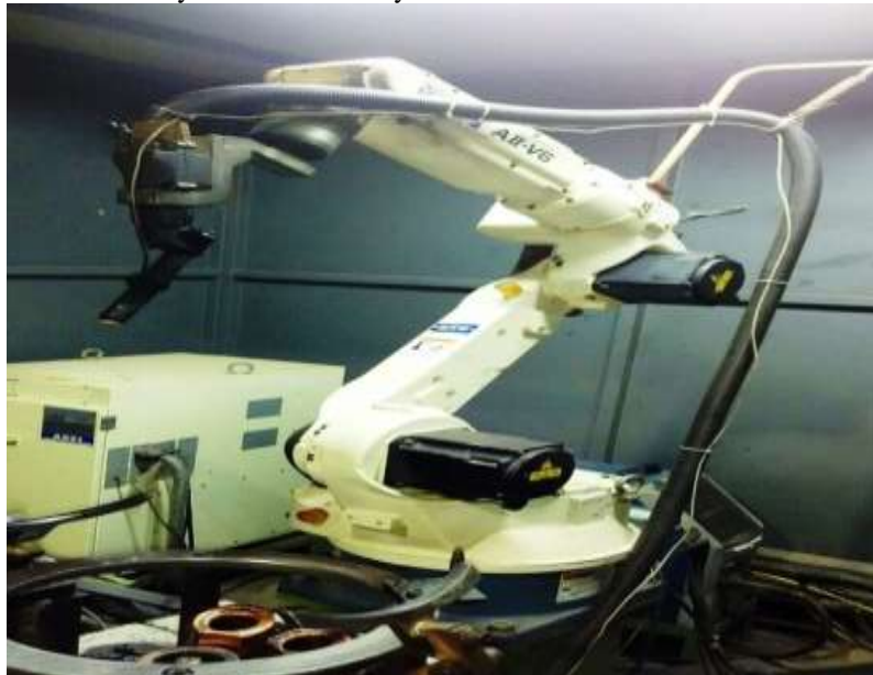
Figure -3.5 Robot OTC AII-V6 for TIG Welding
